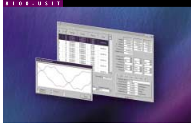
8100-USIT Automatic Meter Calibration Software The 8100-USIT Software configures and controls the Model 8100 to automate testing and calibration of voltage, current, energy, and power meters.
